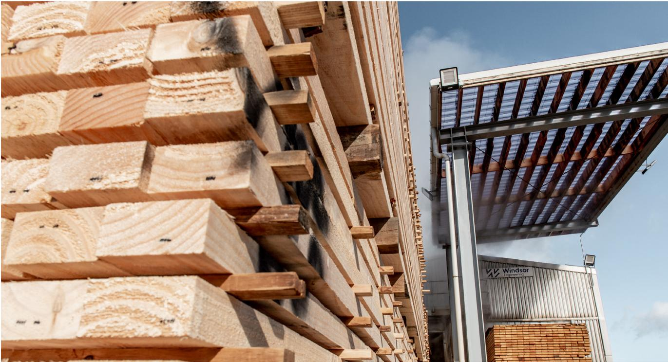
Radiata pine is sourced from sustainably managed forests for the two CHH sawmills at Kawerau and Nelson. The wood is debarked and cut to various product dimensions, maximising the fibre within the log. Subsequent processes include kiln drying to reduce the moisture content and stabilise the timber,
